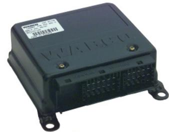
It is a requirement for all WABCO ABS or ABS based systems (EBS) to have the correct startup (End-Of-Line) procedure carried out before the vehicle enters service. This is particularly relevant when retrofits of systems such as Traction Control, or Roll Stability Control, are carried out.
